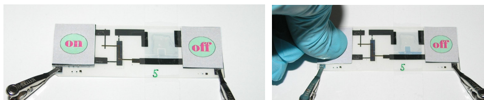
Demonstrator before (left) and after switching on the display element (right).
