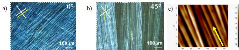
Figure 4. a,b) Polarized optical microscopy images of semiconductor molecule DTT7 on glass substrate; c) AFM images of DTT7 layers on Si/SiO 2 . Yellow arrows: Casting direction.
